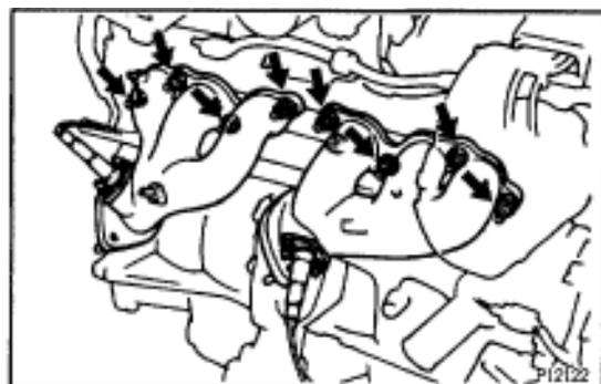
7. REMOVE EXHAUST MANIFOLDS
