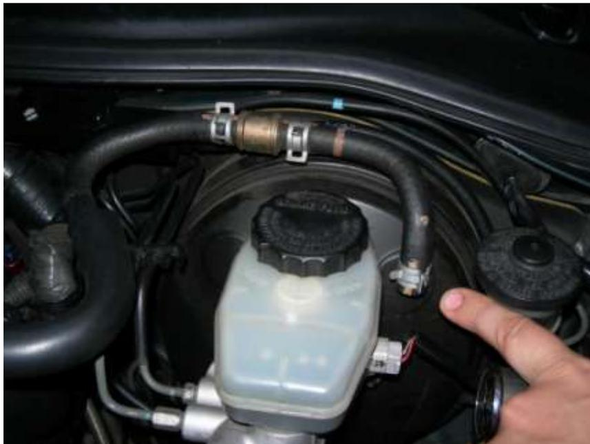
3. Now, notice in the first photo above where the vac line goes into the intake manifold, there is a nipple up there. Simply loosen that nut on top and rotate the nipple towards the firewall such as this:
