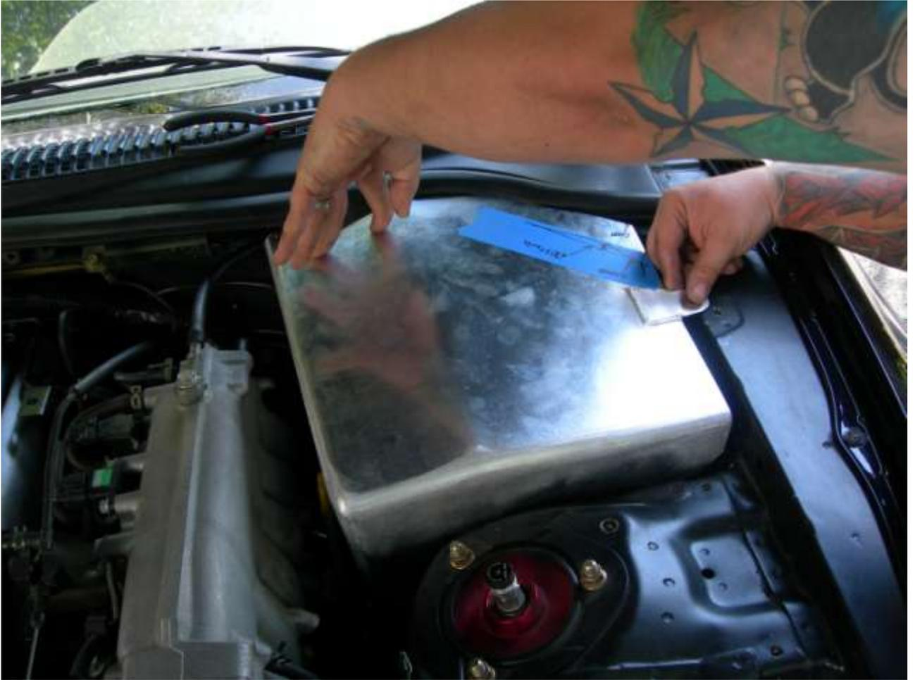
Now pull it over towards the fender and install the bolt in the top of the fender, which, by the way, should be a 12mm bolt which is bigger than the 10mm on the other side:
