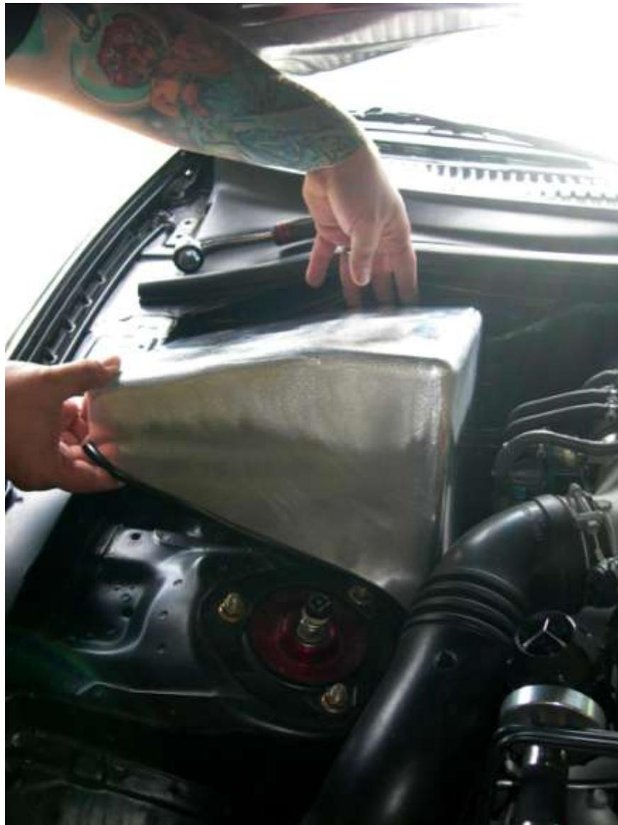
Once it is in place, simply use the bolt hole that is on top of the fender to fasten it in place. It is the only fastener that you need. This side is done !!!! Congrats !!!!
