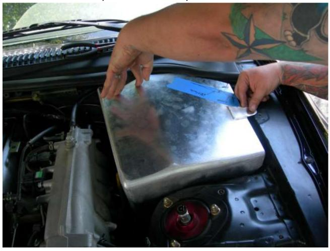
Now pull it over towards the fender and install the bolt in the top of the fender, which, by the way, should be a 12mm bolt which is bigger than the 10mm on the other side:
