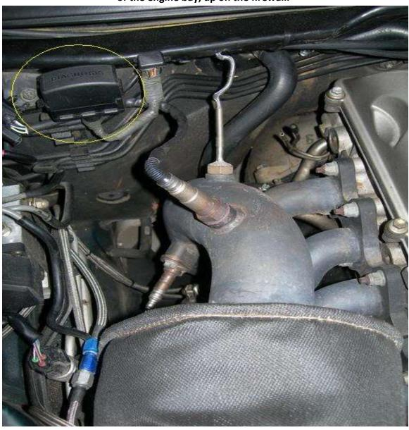
2. Simply pop the diagnostic port off of the bracket, you just need a small flathead screw driver to unclip it. Now, you don't have to remove the bracket if you don't want, but if you want to get rid of stuff in your engine bay, here is how to do it: there are 3 bolts on it, which are in the photo below, simply remove those and pull the bracket off and do what you want with it, I threw mine at my neighbor !!!!
