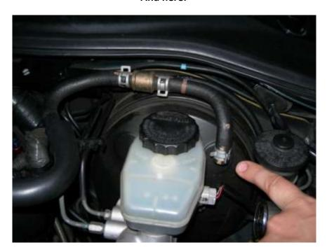
3. Now, notice in the first photo above where the vac line goes into the intake manifold, there is a nipple up there. Simply loosen that nut on top and rotate the nipple towards the firewall such as this:
