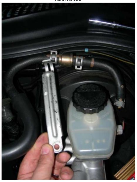
2. Now that that useless bracket is out of the way, and that nut is replaced, you are going to remove the entire vac line, from the booster, all the way to the manifold as seen here:
