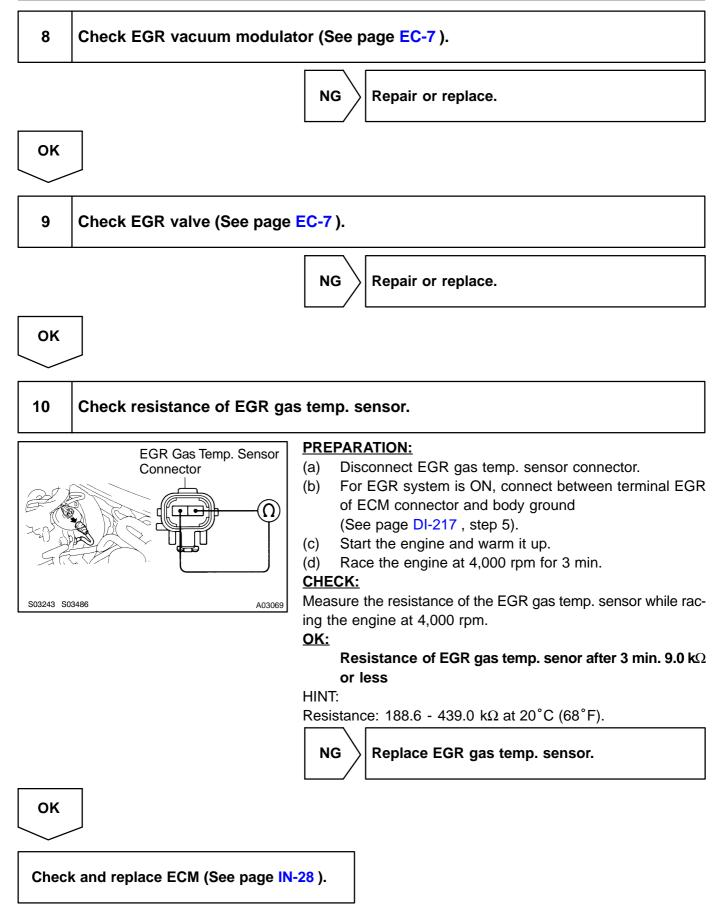
**Exhaust Gas Recirculation Flow Excessive**
