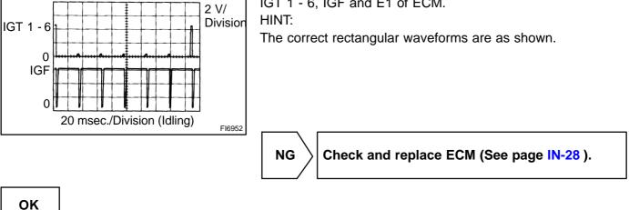
Disconnect igniter connector and check voltage between terminal IGT 1 ~ 6 of
