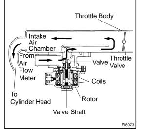
The step motor type IAC valve is located in front of the intake air chamber. Intake air bypassing the throttle valve is directed to the IAC valve through a passage. A step motor is built into the IAC valve. It consists of 4 coils, a magnetic rotor, valve shaft and valve.
