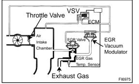
If even one of the following conditions is fulfilled, the VSV is turned ON by a signal from the ECM. This results in atmospheric air acting on the EGR valve, closing the EGR valve and shutting off the exhaust gas (EGR cut-off).
