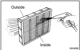
PREPARATION: Remove air filter. CHECK: Visually check that the air cleaner element is not dirty or excessively oily. HINT: If necessary, clean element with compressed air. First blow from inside throughly, then blow from outside of element.
