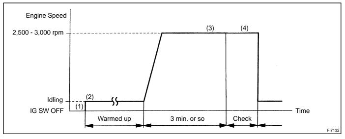
(1) Connect the TOYOTA hand-held tester to the DLC3, or connect the probe of the oscilloscope between terminals OX1, OX2, and E1 of ECM.
