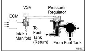
The ECM turns on a VSV (Vacuum Switching Valve) to draw the air into the diaphragm chamber of the pressure regulator if it detects that the temperature of the engine coolant is too high during engine staring.
